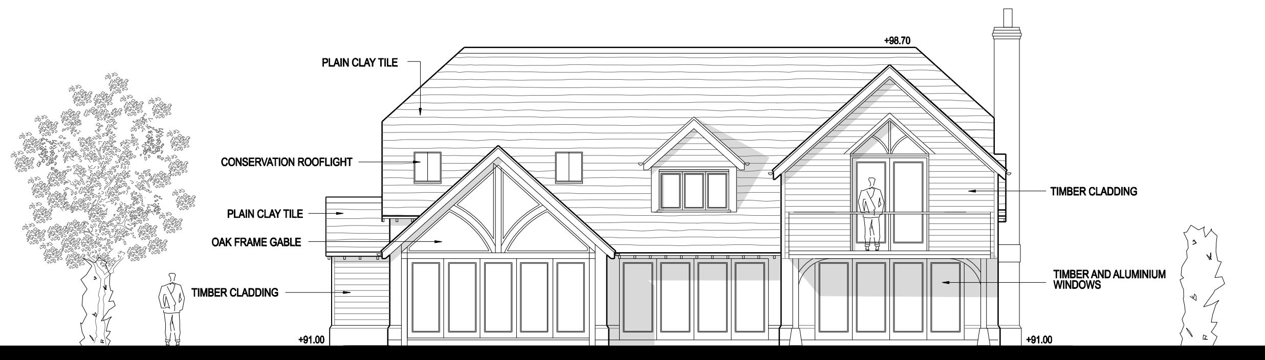
PROPOSED REAR (SOUTH-EAST) ELEVATION
